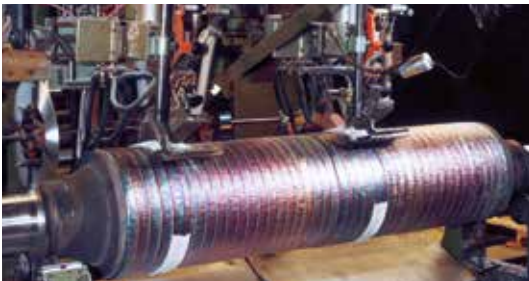
Steelworks - Continuous Casting Rollers (Alloy 13Cr6Ni2Mo) Soudotape 430 L + Record RT 168
