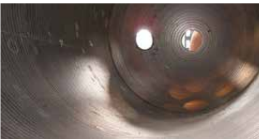
Pressure Vessel (Stainless steel alloy 347) Soudotape 24.12 LNb + Record EST 136
